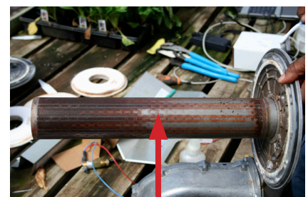
Burner & door assembly—prior to fiberboard installation
