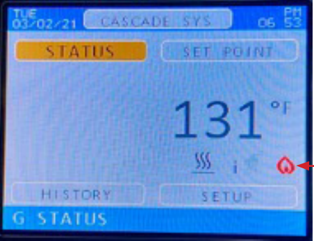
Flashing icon indicates demand in process (iDHW):
